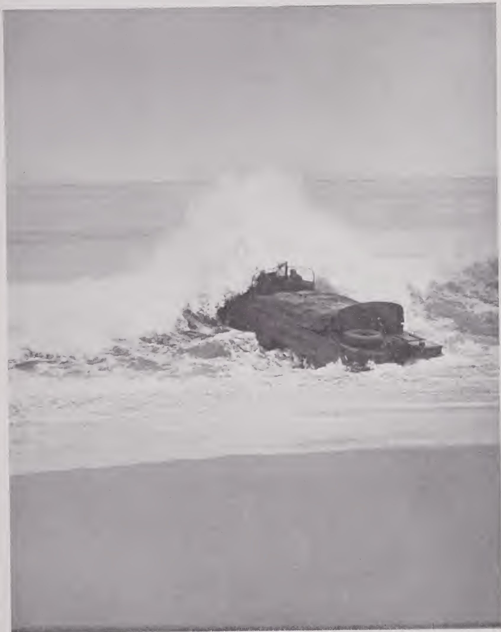
The DUKW, the "truck that goes to sea," developed as an amphibian for operation on land and water and for the zone between—surf and treacherous sand.
